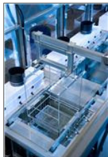
Involving more than just a tank, an effective and productive ultrasonic cleaning system needs to address maintenance of bath quality through filtration or periodic replenishment, rinsing methods for removing cleaning residues, and part drying.
